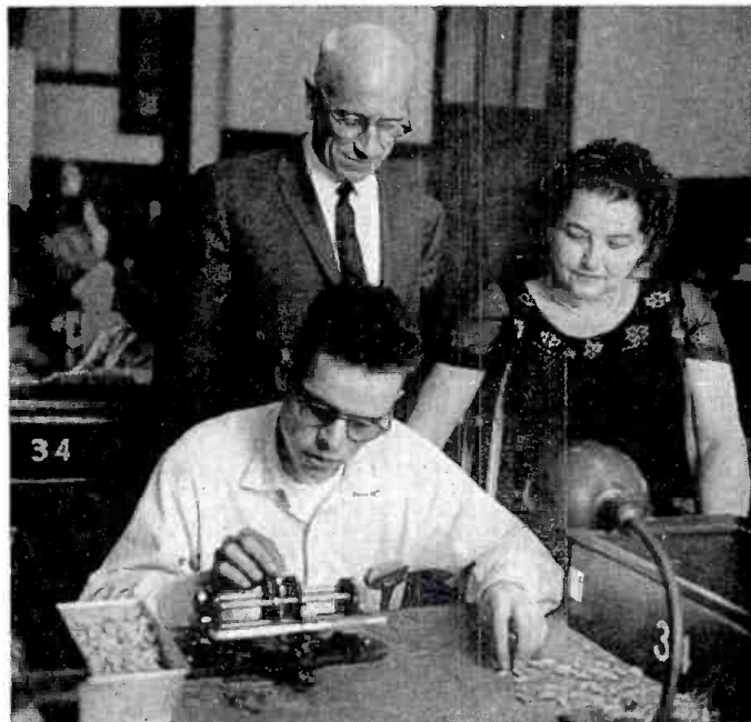
Over $140 Million was spent by Western Electric with New England suppliers during 1962. One such company, Pace Industrial Corp. of Portsmouth, New Hampshire, is operated entirely by handicapped people. The firm produces a device used to prevent overloading in carrier switching equipment. Below, President Dorothy Pace and W.E. Buyer Les Currier (left), look on as Frank Jolley, a Pace employee, connects the leads on one of these units.
